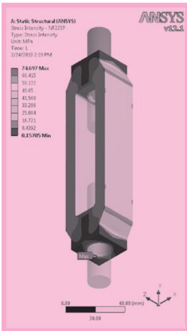
Stress Levels in Turnbuckle calculated using ANSYS.
